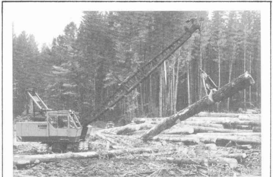
Rope Crane Loader: available in limited size range, not suited to large numbers of log sorts, and requires highly skilled operators. Effective on small landings, poor surfaces, and at trailer off-loading. Has good lift height and long machine life.
