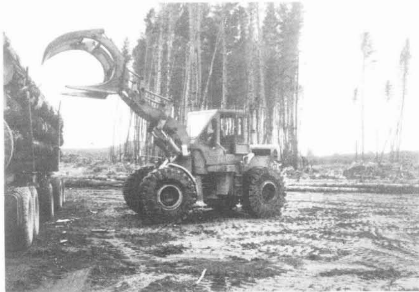
Rubber-tyred front-end loader: needs larger landings with good surfaces. Has good versatility and mobility and is effective for working large numbers of sorts. Is a very common type of machine and is available in a large range of sizes.
