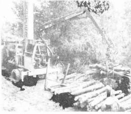
FIG.3 Cranab stacking short-pulp into multi-lift cradles.
