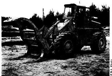
Possible improvements in equipment utilisation and system production rate could be obtained if the loader was used to pull logs aside from underneath the hauler spar. This would reduce skidwork interruptions to the hauling phase thereby increasing hauler production and, correspondingly, loader utilisation and production. The ability of the loader to perform the rouse this task would a need evaluation. this task would however
