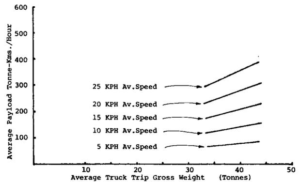
FIG.4 Graph showing effect of gross weight on payload tonne-kilometres per hour.
