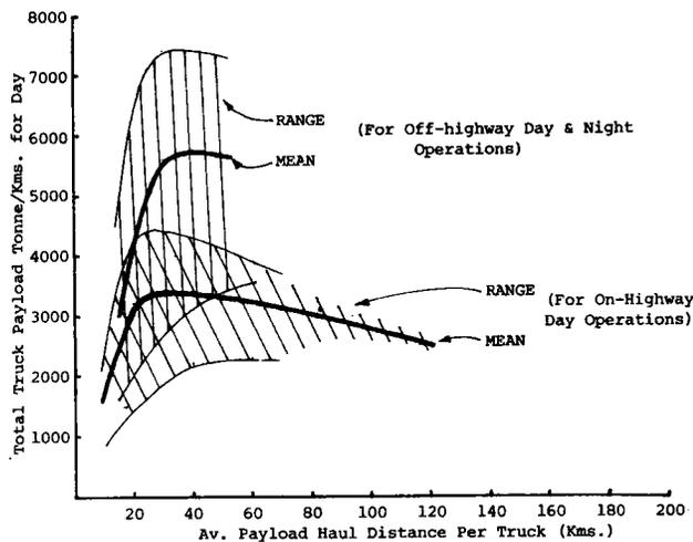
FIG.1 Graph showing effect of haul distance on payload tonne-kilometres per day.
