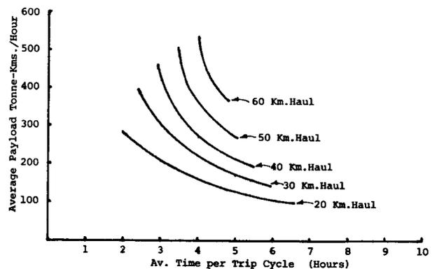
FIG.2 Graph showing effect of trip cycle time on payload tonne-kilometres per hour. (For 300 h.p., 45 tonne gross weight NZFP off-highway trucks.)
