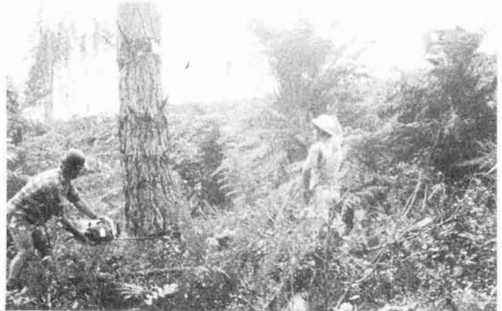
Method 2. Tractor out of striking range with faller and signalman at butt.
