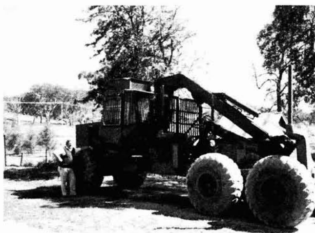
Figure 3 - Kockums 85-33 Forwarder now used as a training machine by ERFIC in Tumut, New South Wales
