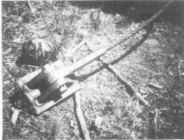
Figure 3 - Soil toggle fabricated by U.S. Forest Service.
