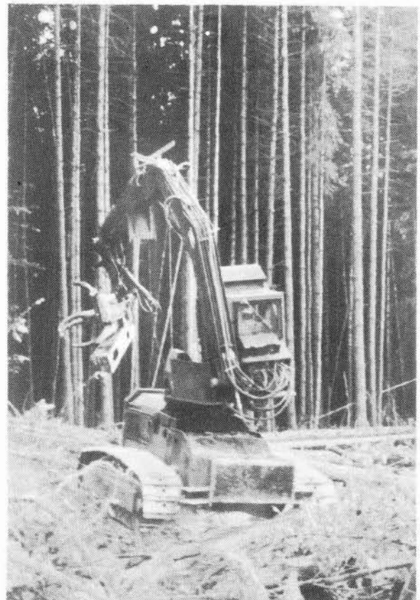
Figure 1 - Timbco 2518 with Weyerhaeuser W-34 Feller-Director head
