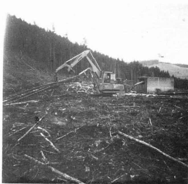
Figure 2 - Second swing moves the logs closer to the landing
