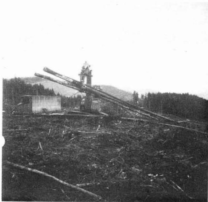
Figure 1 - Swinging logs from the stump with a hydraulic loader
