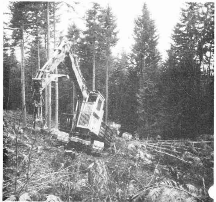
Figure 4 - Loader working a 40% sideslope
