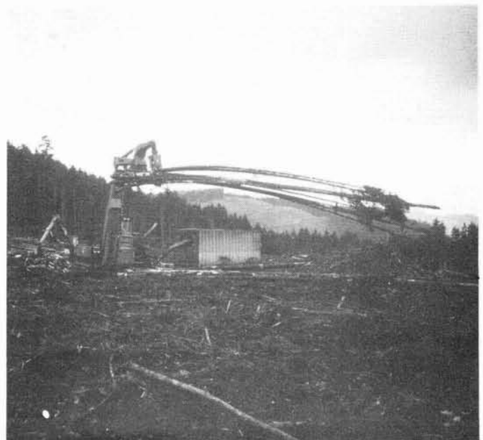
Figure 6 - Live heel and grapple is recommended for swinging
