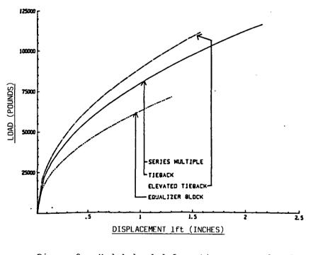
Figure 2 - Model load-deformation curves for four rigging configurations. The curves end at the load where system failure occurs
