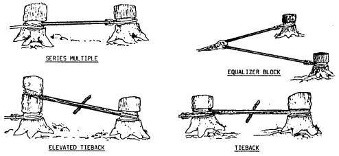
Figure 1 - Multiple anchor rigging configuration
