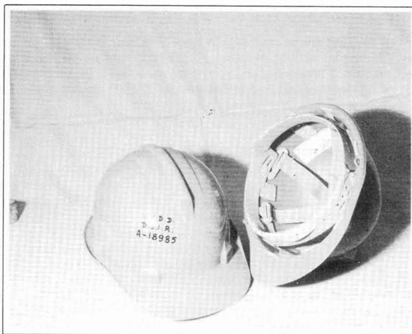
Fig. 1 - The shell and inner harness support system of an industrial safety helmet
