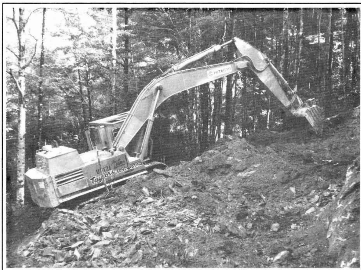
Fig. 1 - Hitachi UH121 Excavator cutting down to grade from a pilot track.
