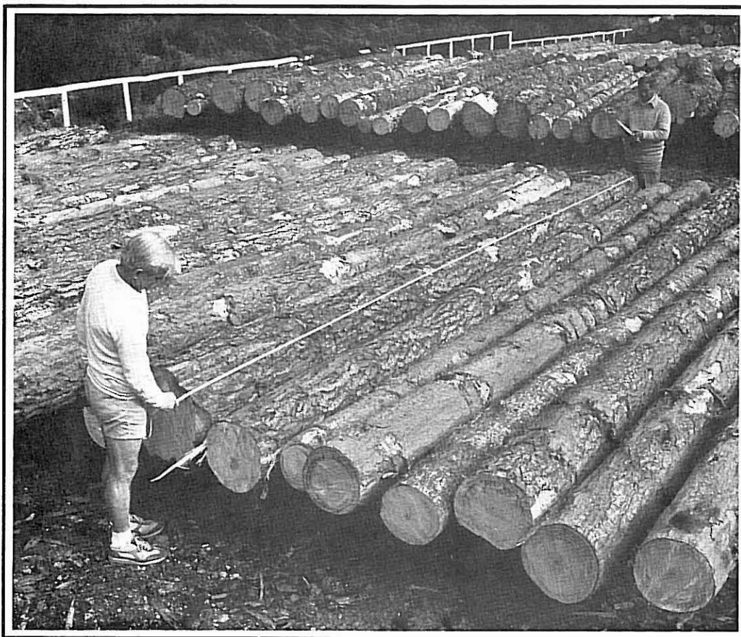
Fig. 3 - Measurement of sample load to obtain volume
