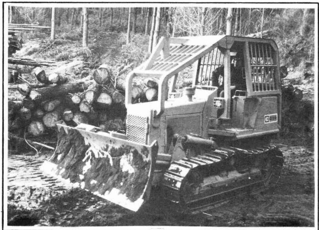
Fig. 1 - Caterpillar D3B ready for skidding
