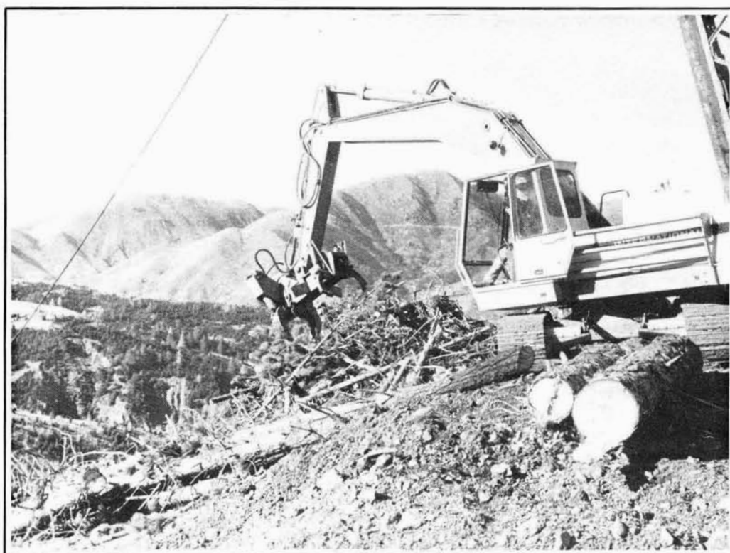
Fig. 1 - 640 HD International fitted with delimber boom and grapple shear.
