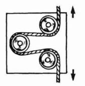
• a wear test for 400 cycles, then the tensile pull test to destruction
