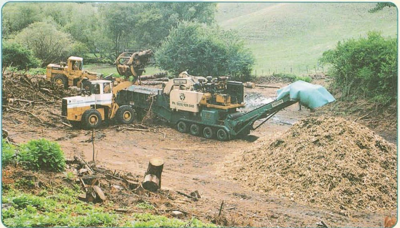
*Figure 1 - Wastepro hog being loaded with logging landing residue and producing boiler fuel*
