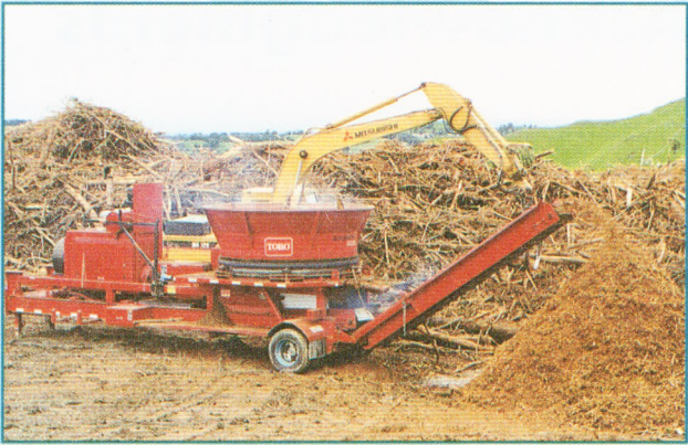
Figure 4 - Tubgrinder processing logging residue into boiler fuel
