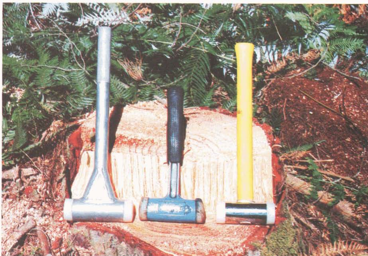
Figure 1 (from left to right) - Scorpro shot filled hammer, standard Thorace shot filled hammer, modified Thorex hammer
