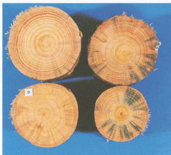
Figure 1 - Log ends showing sapstain wedges
