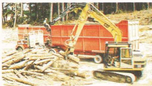
Figure 1 - Foreground, Cat 311 excavator, loading a bin truck from a pile of reject wood. The truck is a 6x4 with a three-axle trailer fitted with a self-loading crane. Obscured at the rear is an 8x4 bin only truck with a four axle trailer
