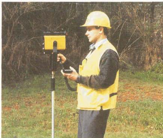
Figure 1 - Criterion 400 Survey Laser with a data recorder
