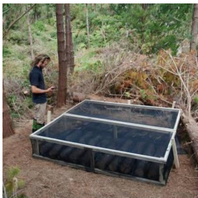
Figure 2. Alwin Sky taking a GPS co-ordinate at Mahinapua Forest, West Coast. Note the paired design with complete insect exclusion at front, and an open-sided mesh screen at rear.
