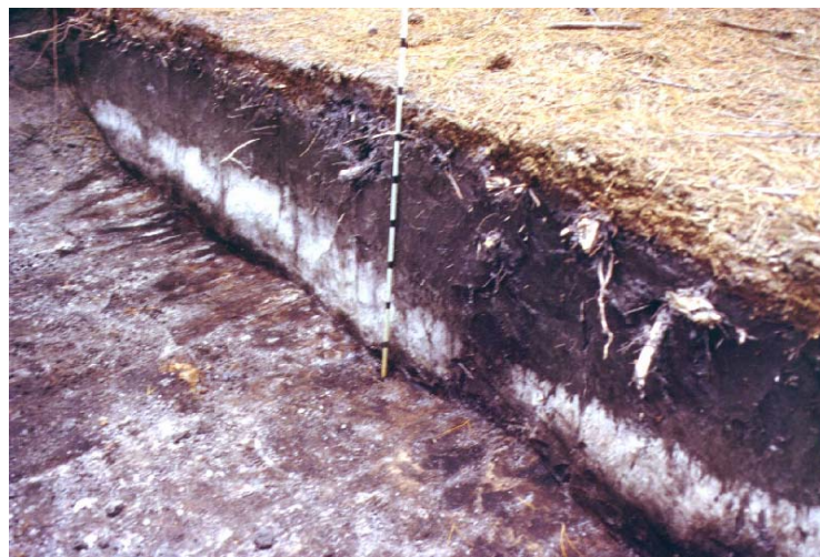
Figure 17. Soil profile and tree rooting pattern for a ripped plot for Trial AK578/1, showing negligible observable effects of ripping. Note that pine tree roots are limited to the topsoil horizons. The centre of the trench is aligned with the tree row. Scale marker is in 10-cm increments.
