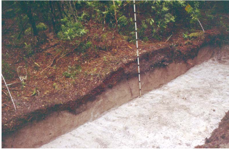
Fig. 18 Soil profile and tree rooting patterns for a ripped and bedded plot for Trial AK662. Note that tree rooting is limited to the topsoil and was unable to penetrate the underlying densipan. The centre of the trench is aligned with the tree row. Scale marker is in 10-cm increments.
