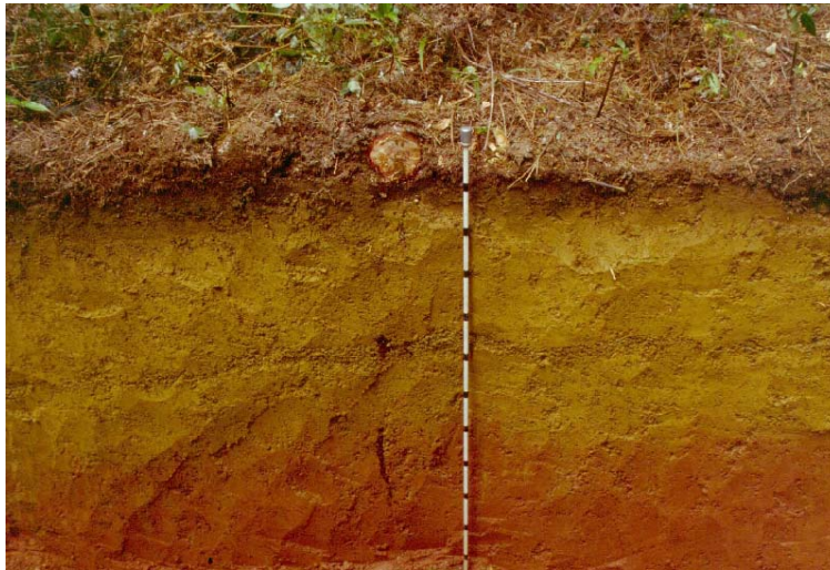
Fig. 16 Soil profile and tree rooting pattern of a ripped plot for trial AK578/2, showing negligible observable effects of ripping. Note the gravel layer at about 40 cm. The centre of the trench is aligned with the tree row. Scale marker is in 10-cm increments.
