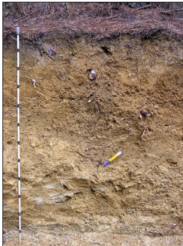
Fig. 7 Close-up showing roots in a U-shaped loosened zone down to about 70 cm (marked by the pen) for ripped 2 site. Scale marked in 10-cm increments.
