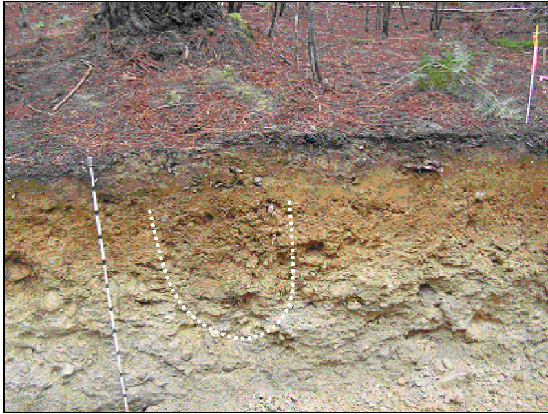
Fig. 4 Trench soil profile for ripped 1 site. Note roots in the U-shaped loosened ripped zone (to about 65 cm, outlined by the dotted line) to the right of the scale marker.
