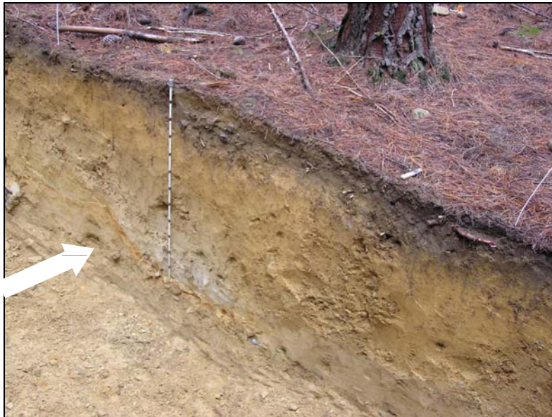
Fig. 3 Trench soil profile for the unripped Control plot showing large roots confined to the Ah horizon. The pale zone with iron-pan at base (at 1–1.2m depth, arrowed) is a localized, saucer-shaped gleyed zone. Scale marker is in 10-cm increments in all photographs and the small white flag stems mark the ends of the 3-m transect.
