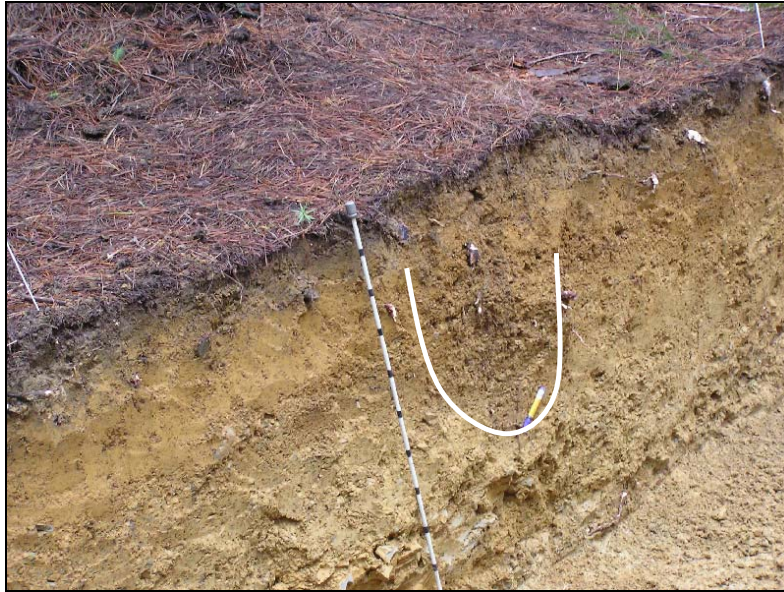
Fig. 6 Trench soil profile for ripped 2 site. Note roots in the U-shaped loosened ripped zone (to about 70 cm, dotted line) to the right of the scale marker. The blue pen tip points to the bottom of the loosened zone. The white flag stems mark each end of the transect.
