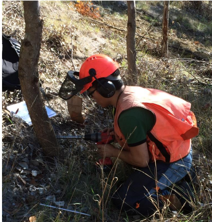
Figure 1. Extracting a core from an E. bosistoana tree using a light-weight, battery-powered tree corer developed for the New Zealand School of Forestry.
