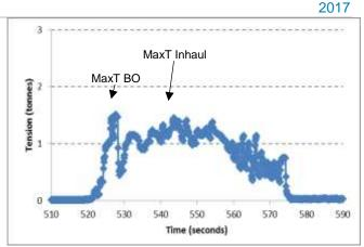
Figure 5: Typical cycle showing tensions measured during breakout and inhaul phases.
