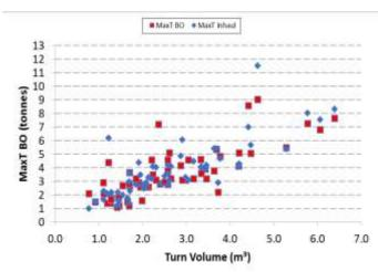
Figure 6: Relationship between maximum tension during breakout and inhaul, and turn volume.
