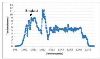
Figure 9: Breaking out larger payload (4.6 m<sup>3</sup>) out of pile with high difficulty rating.
