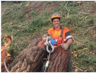
Figure 4: Wireless Load Shackle attached to choker and mainline swivel dee at Study Site 1.
