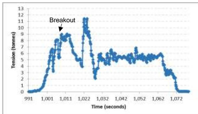
**Figure 9: Breaking out larger payload (4.6 m<sup>3</sup>) out of pile with high difficulty rating.**
