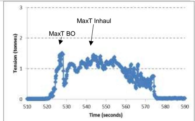
**Figure 5: Typical cycle showing tensions measured during breakout and inhaul phases.**
