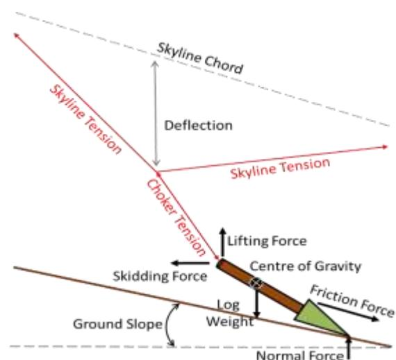
**Figure 1: Forces acting on a partially suspended log (adapted from Mifflin, 1982).**
