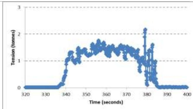
**Figure 8: Easy break-out and in-haul, but data shows shock loading event up at landing.**
