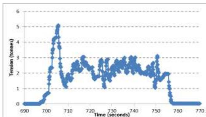
**Figure 7: Higher breakout force but smooth inhaul.**
