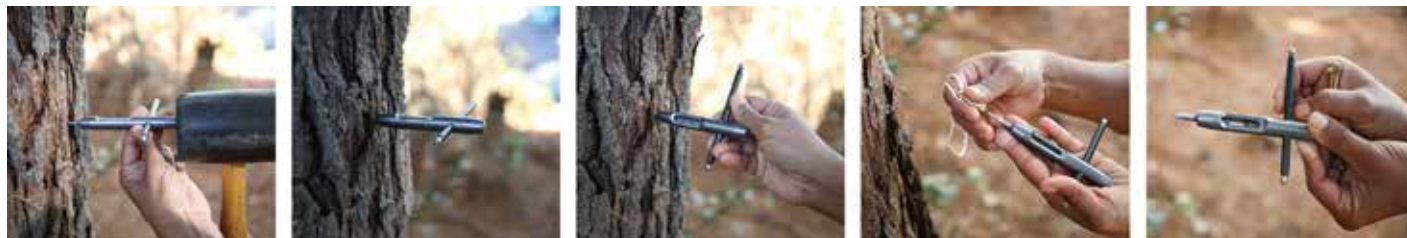
Microcore sampling using a Trephor tool.
