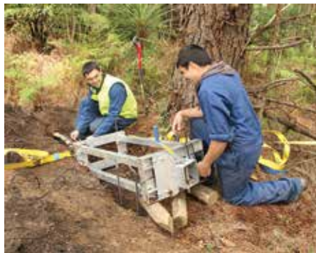
University of Sassari (Italy) researchers conducting root pullout tests on 23-year old radiata pine trees near Gisborne.
