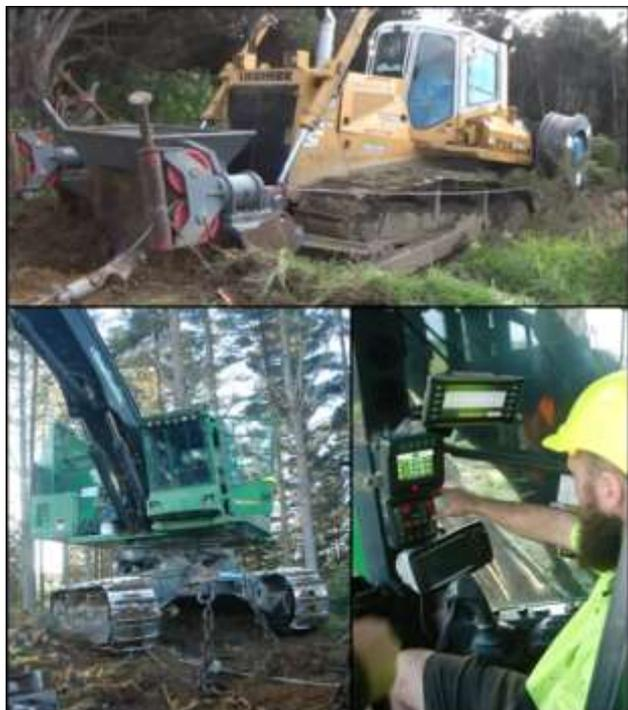
Figure 1: Remote Operated Bulldozer (ROB) system.
