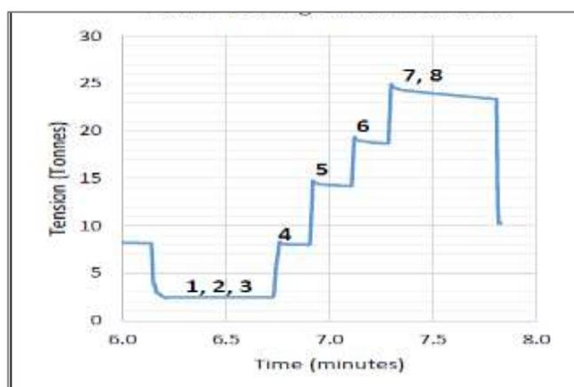
**Figure 15: Falcon winch power setting calibration test, with winch settings 1-8 indicated by bold text.**
