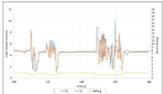
**Figure 13: Tractionline rope tensions indicating winch setting, with shock loads above base tension.**
