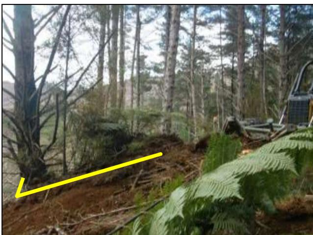
**Figure 9: ROB winch-assist machine set-up, with yellow line showing ropes wrapped around tree.**
