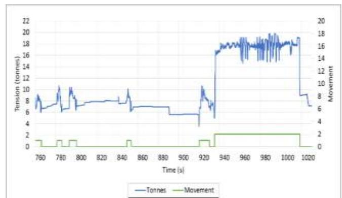
**Figure 14: Falcon rope tension when moving downhill then uphill, with shock loading above base tension.**
