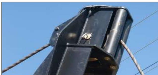
Figure 4: Load pin sheave for monitoring tension.
