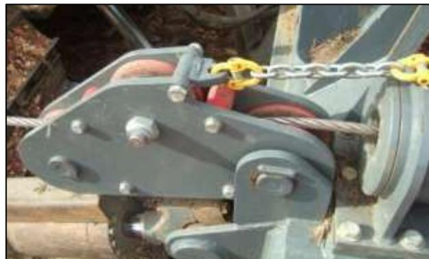
Figure 6: Tension monitor sheaves on the ROB system.
