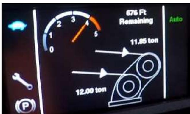
Figure 5: Tractionline tension display system.
