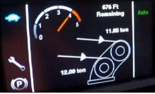
Figure 5: Tractionline tension display system.
