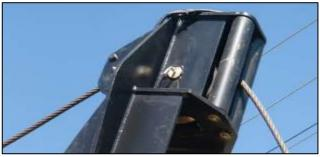
Figure 4: Load pin sheave for monitoring tension.
