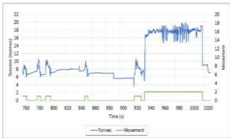
Figure 14: Falcon rope tension when moving downhill then uphill, with shock loading above base tension.
