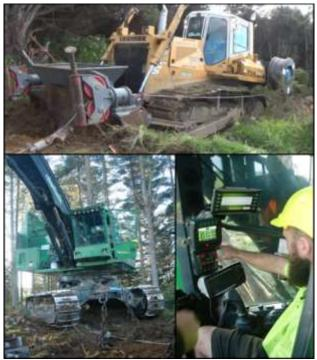
Figure 1: Remote Operated Bulldozer (ROB) system.
