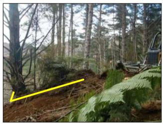
Figure 9: ROB winch-assist machine set-up, with yellow line showing ropes wrapped around tree.
