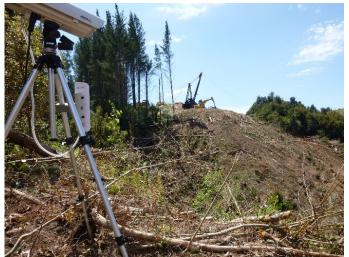
Figure 1. The first prototype comprised a hauler camera, a tail hold camera, a cutover camera (pictured) and a hauler cab display.
