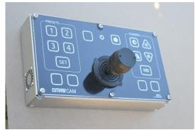
Figure 4: CutoverCam control panel featuring an industrial joystick and touch screen controls
