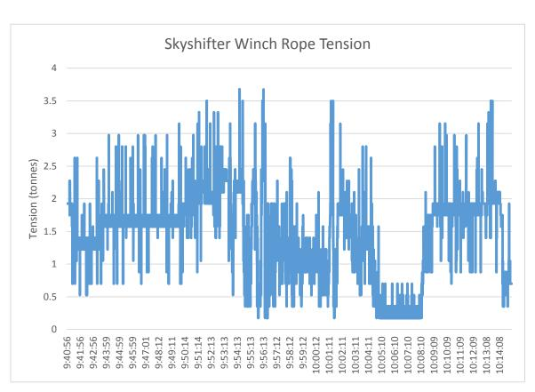
Figure 18: Actual tension monitor readings of right hand winch rope during movement of the Skyshifter
