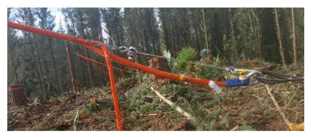
Figure 15: Tightening the adjustable synthetic guy ropes with a light weight "cumalong".
