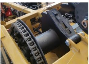
remote control and can withstand 30 tonnes of skyline tension. Due to the length of the carriage, the winch drums did not need a rope spooling mechanism. The winch drums have a 7-tonne line pull, almost double the design parameter. The selected design did allow the use of synthetic winch ropes, which weren't a design parameter, but it became evident early in the design process that synthetic winch ropes were going to be a key requirement to aid quick and easy setup.
