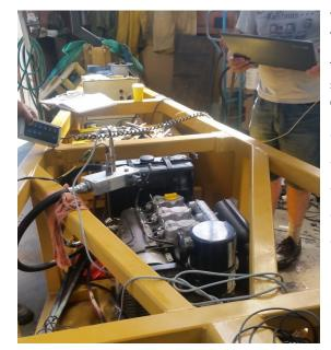
Figure 4: Programming the hydraulics and engine management system
