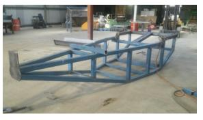
Figure 3: Skyshifter frame during construction
