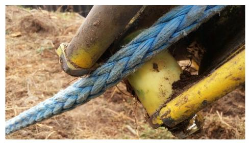
Figure 11: Sharp angles anywhere synthetic rope can touch must be avoided (both on the carriage and when the winch lines are extended, including stumps).
