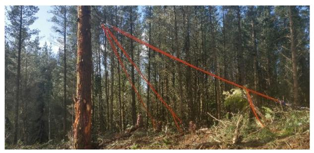
Figure 14: Elevated anchors guyed with adjustable synthetic rope
