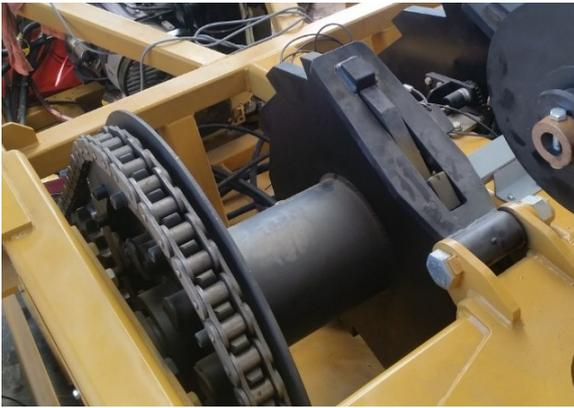
**Figure 2: Skyshifter winch assembly**
