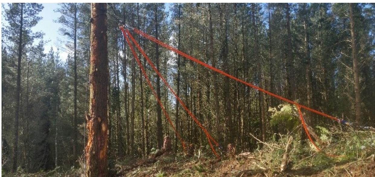
**Figure 14: Elevated anchors guyed with adjustable synthetic rope**
