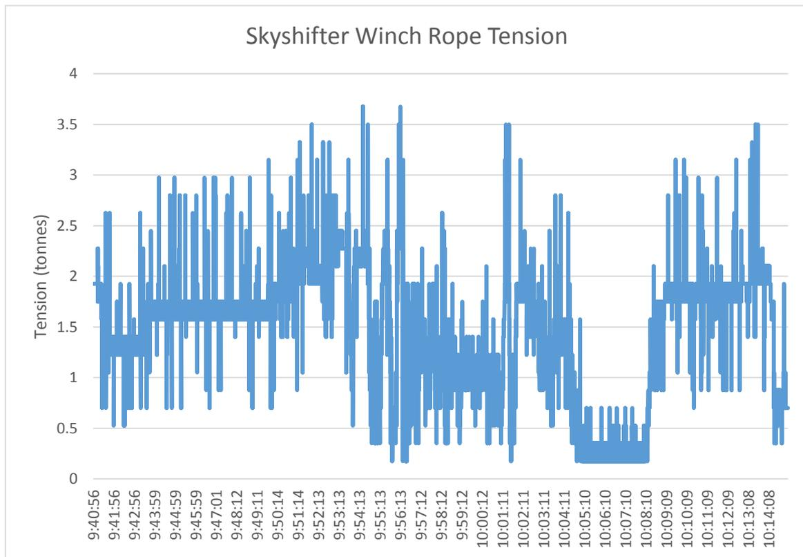
**Figure 18: Actual tension monitor readings of right hand winch rope during movement of the Skyshifter**
