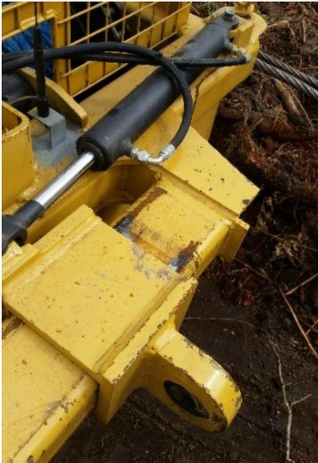
**Figure 6: Skyline balancing mechanism to keep Skyshifter level with varying winch rope tensions**
