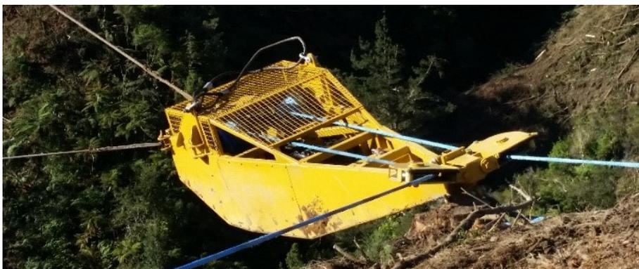
**Figure 9: Skyshifter setup on a 32mm skyline**
