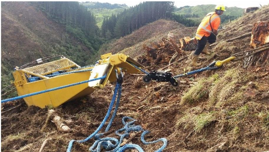
**Figure 8: Skyshifter in position just prior to being lifted into working position with the skyline**
