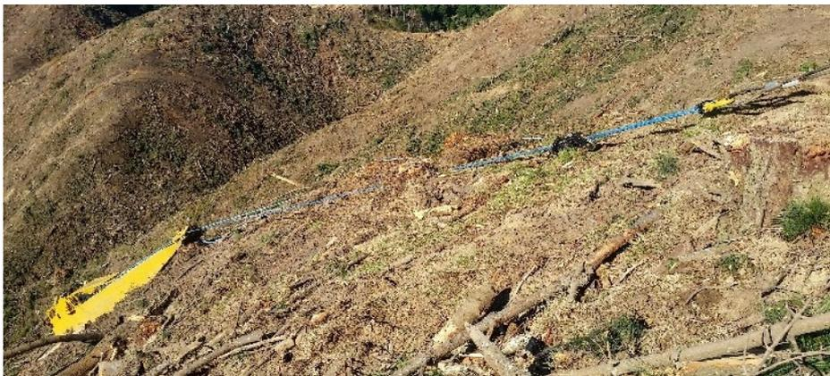
**Figure 10: Poor deflection at the backline made shifting the Skyshifter very difficult.**
