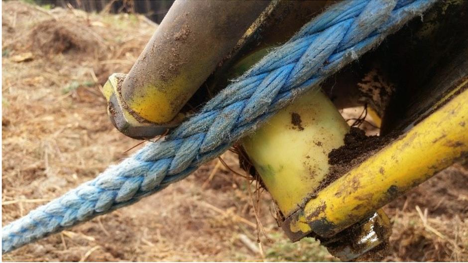
**Figure 11: Sharp angles anywhere synthetic rope can touch must be avoided (both on the carriage and when the winch lines are extended, including stumps).**
