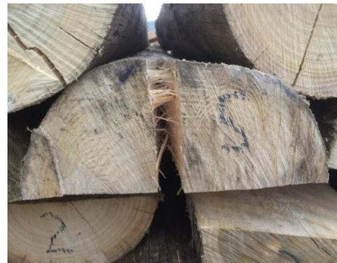
The results of the mechanical testing showed that the *E. nitens* OEL (photo of product below) achieved the strength and stiffness properties of the New Zealand structural grade SG12. The process will need fine tuning for *E. nitens* as standard (*radiata*) set-ups were used for finger jointing and gluing.
