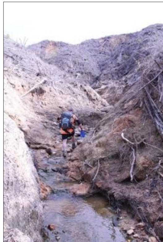
Channel scour to bedrock. Note 'clean' lower slopes, suggesting erosion by debris flow.
