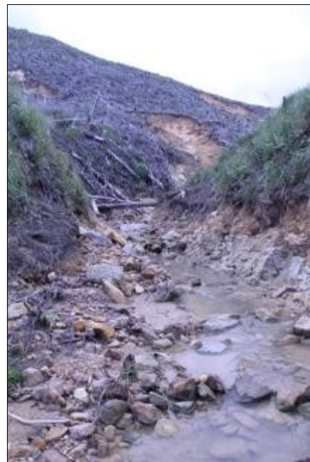
Riparian and lower slope failures exposing bedrock. Note scour in channel to bedrock and 'flow' line RHS.
