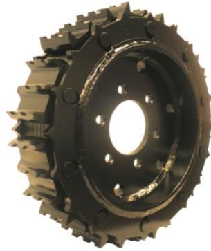
Figure 5. Moipu outer feed rollers similar to the one above and manufactured by Moisio Oy in Central Finland were included in the Australian debarking feasibility trial.
