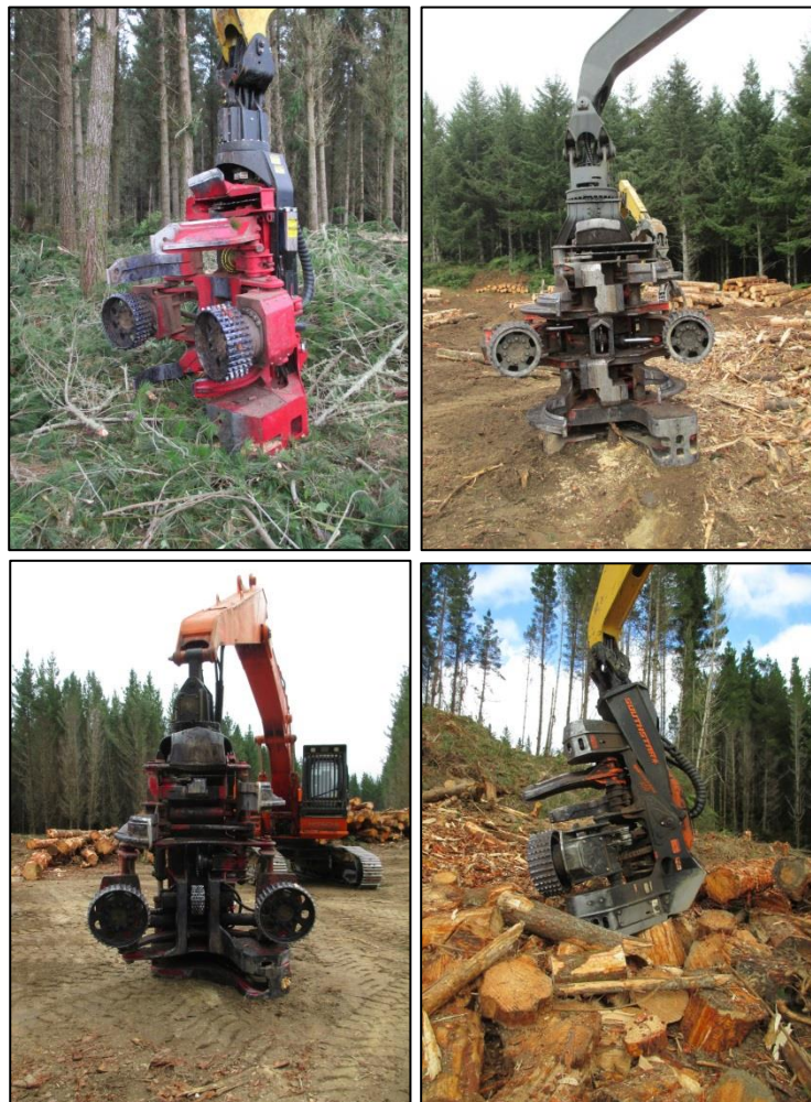
Figure 3. Processor heads which will be compared in the third milestone period on the basis of bark removal. From top left and clockwise: Waratah 625 (4-knife), Woodsman Pro 800 (4-knife), SouthStar (2-knife), and Waratah 626 (2-knife)
