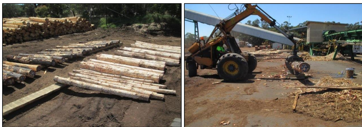
Figure 3. Logs used in Australian Spring drying rate trial (left) and log being placed on weight scales (right).
