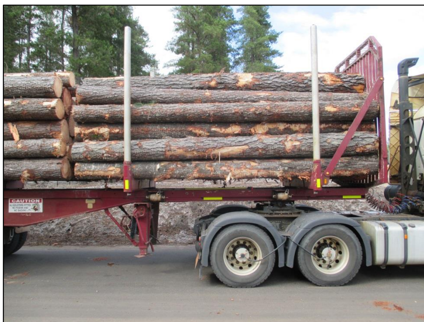
Figure 1. Logs arriving at Wespine mill in Western Australia for the Autumn Bark Loss Benchmarking Study. Also note the headboard fitted to the front of the truck to stop logs sliding forward.
