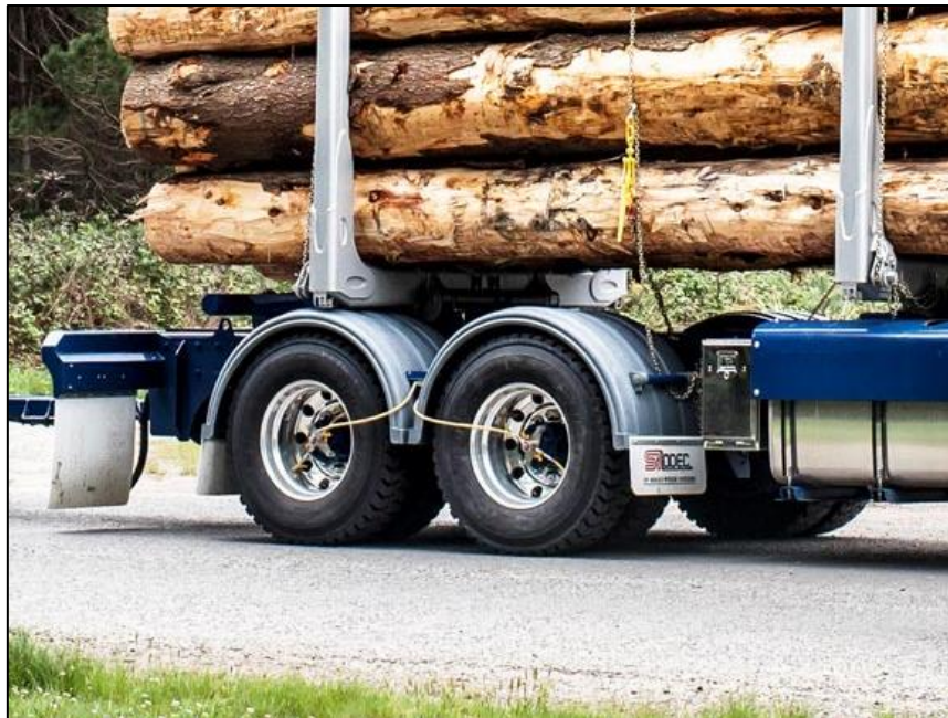
Figure 7. Load securement of debarked logs during transport has been identified as a potential risk in the preliminary review of safety
