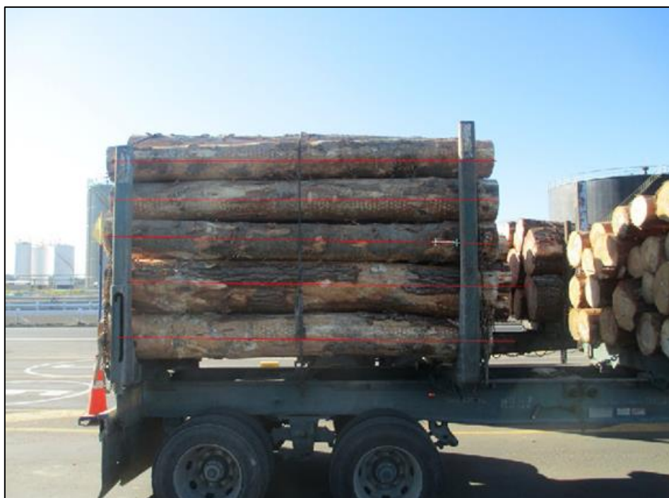
Figure 2. Image of load of logs with lines overlaid in preparation for measurement of bark loss using the line intersect method.
