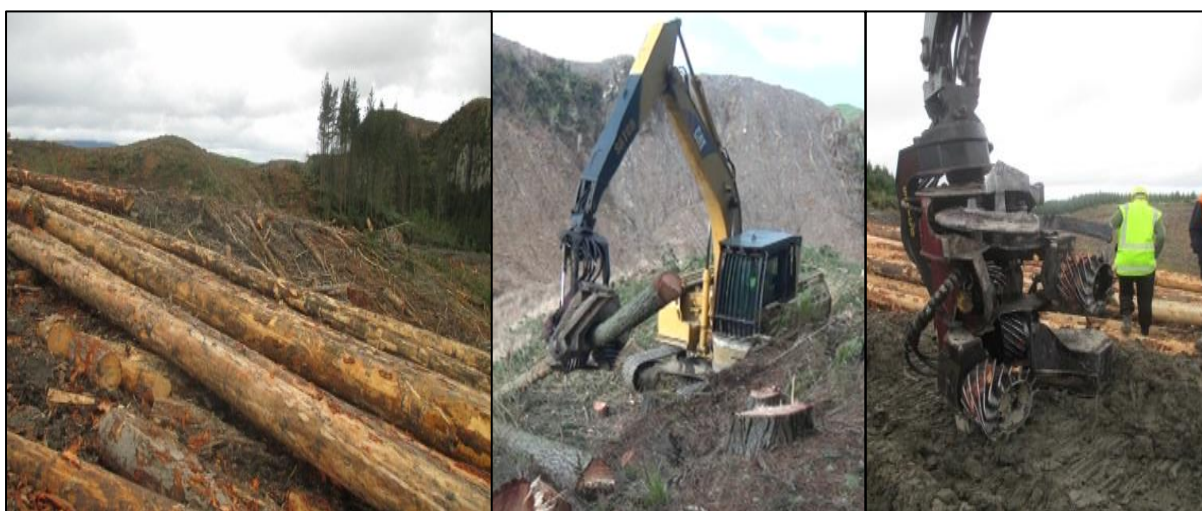
Figure 6. Small almost fully debarked stems (left), Caterpillar excavator with SATCO head (centre), 22 inch SATCO eucalypt debarking head (right)
