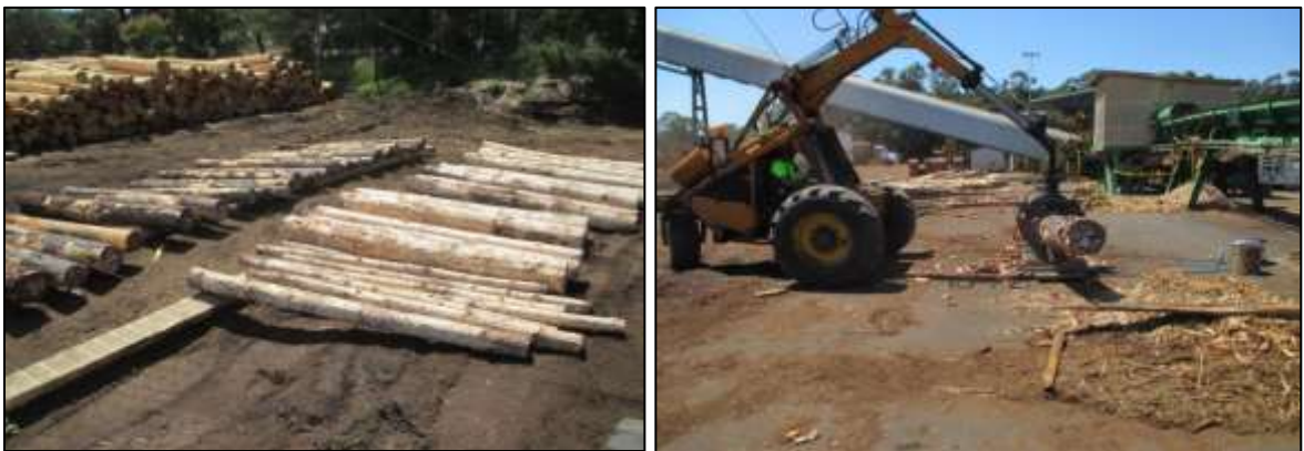
Figure A1.2. Logs used in Australian Spring drying rate trial (left) and log being placed on weight scales (right).
