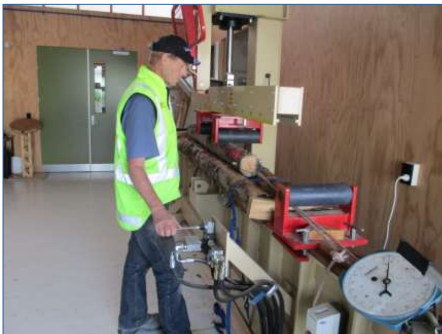
Figure 2. Test bed for measuring static coefficient of friction of Pinus radiata logs with and without bark present.
