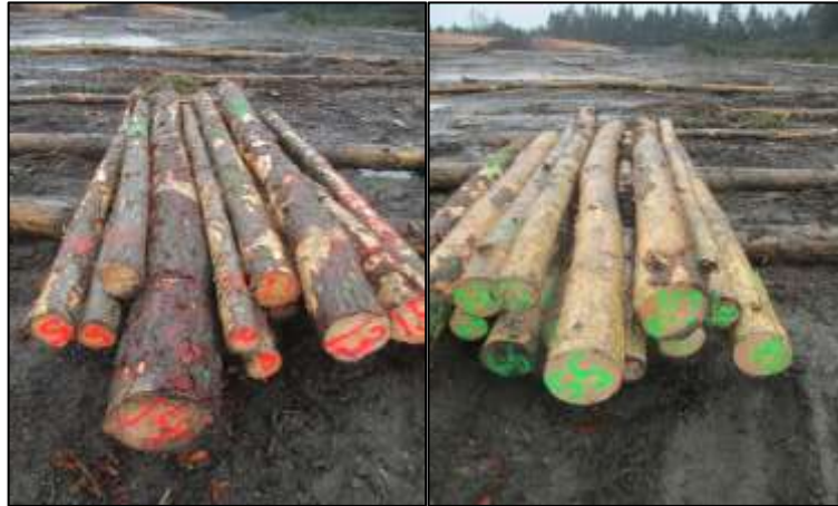
Figure A1.3. Logs with bark largely intact (left) and with bark largely removed (right) in New Zealand Spring drying rate trial.
