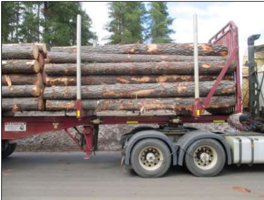
Figure A3.1. Logs arriving at Wespine mill in Western Australia for the Autumn Bark Loss Benchmarking Study. Also note the headboard fitted to the front of the truck to stop logs sliding forward.
