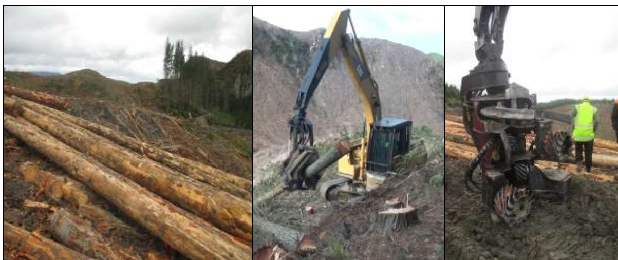
Figure A1.5. Small almost fully debarked stems (left), Caterpillar excavator with SATCO head (centre), 22 inch SATCO eucalypt debarking head (right)
