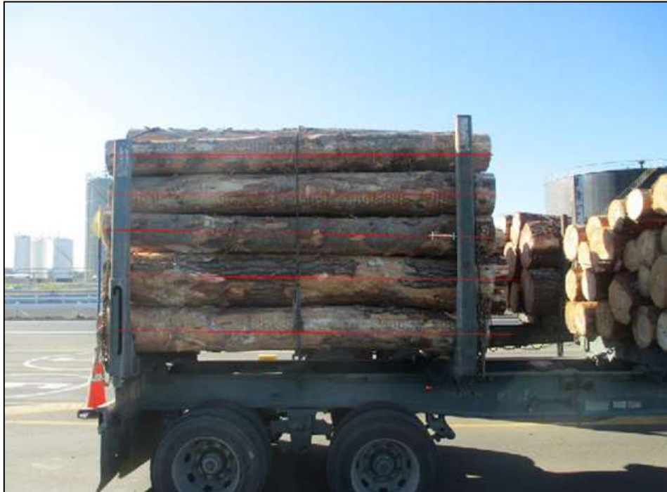
Figure A1.1. Image of load of logs with lines overlaid in preparation for measurement of bark loss using the line intersect method.
