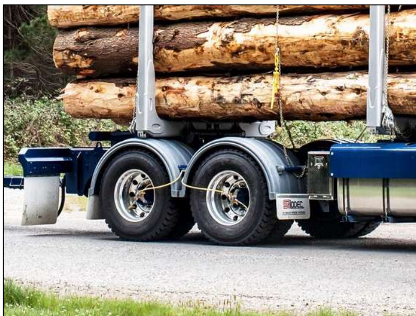
Figure A1.6. Load securement of debarked logs during transport has been identified as a potential risk in the preliminary review of safety
