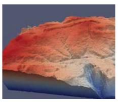
Micro-terrain model extracted at 0.2 m resolution from LiDAR.
