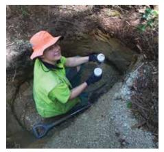
Loretta Garrett installing resin lysimeters into a soil pit in the Timberlands biuret trial.
