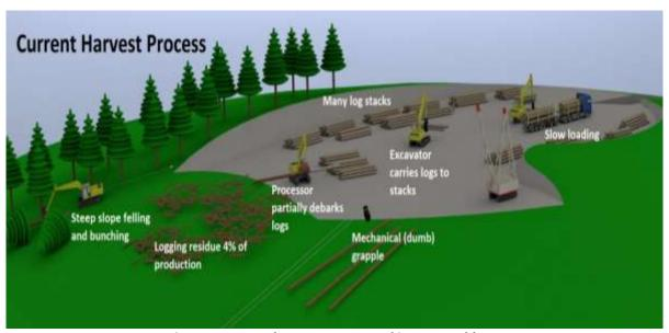
Figure 1: Current harvest process and issues to address
