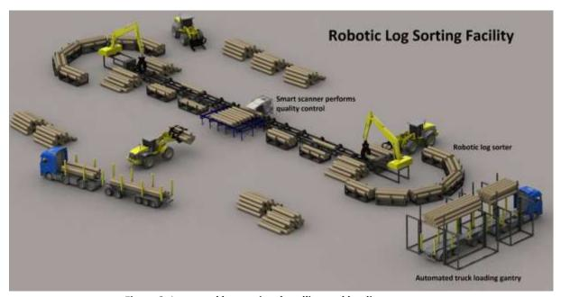
Figure 3: Improved log sorting, handling and loading processes
