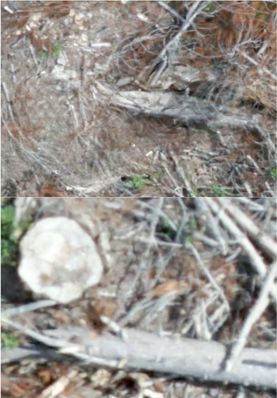
Figure 17: Example of image ghosting from poor matching during orthomosaic generation (top). The bottom panel shows the typical level of detail achieved across most of the site from imagery with a GSD of 0.7 cm/pixel.
