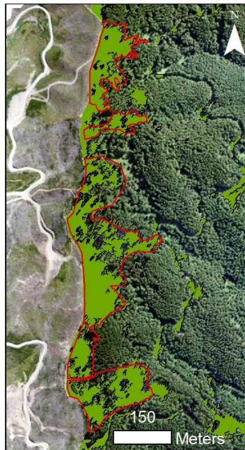
Figure 4: Results from Mahlanobis classification of standing and wind-thrown forest. Approximately 10 ha of damaged forest was identified.
