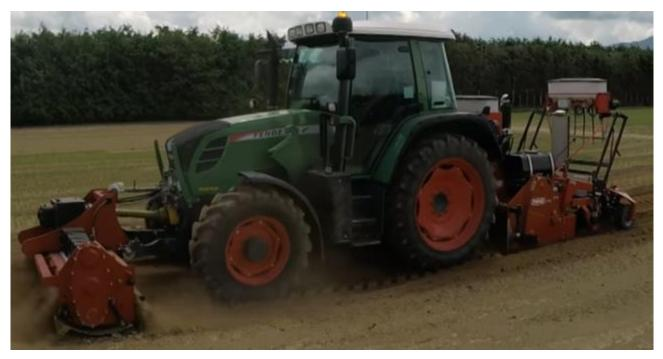
*Figure 1* Example of a tractor equipped with a GPS / radar driven unit that enables precision planting in the seed beds. Although currently occupied, the tractor can operate autonomously.
