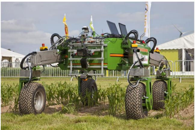
Figure 3 Example of an autonomous platform for conducting operations on plants within the seed bed level
