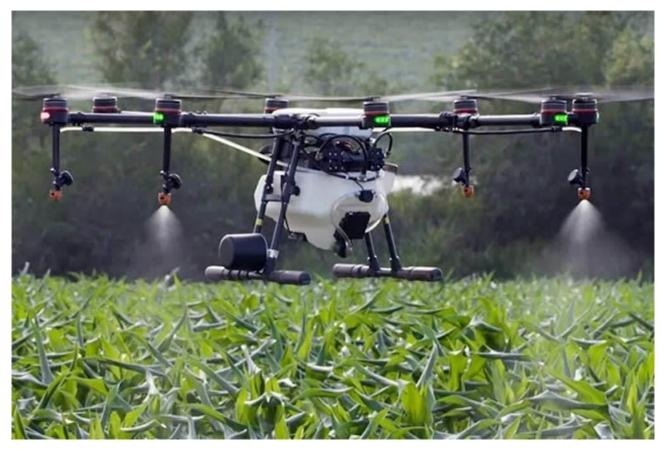
Figure 4 Precision application of agrochemicals using a drone delivery system
