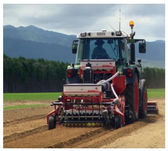
**Figure 2** The leading module (obscured) forms the bed, while the modules following the tractor plant the seed, with additional options to add a treatment at planting. All modules are mounted on lateral actuators that precisely maintain the position of the modules relative to the seed bed being formed.
