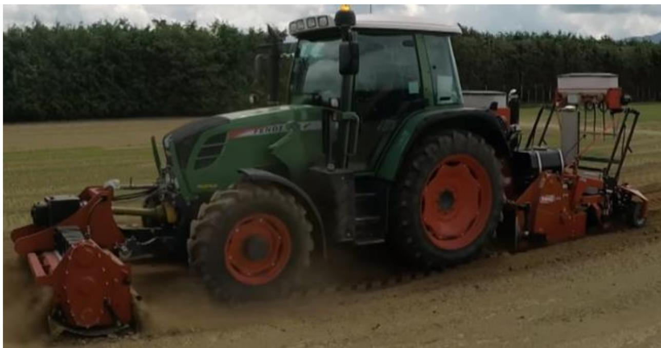
**Figure 1** Example of a tractor equipped with a GPS / radar driven unit that enables precision planting in the seed beds. Although currently occupied, the tractor can operate autonomously.
