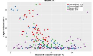
Heartwood of 7 year-old NZ grown *E. bosistoana*, on average, met the performance of a class 2 (aboveground) rated species. This can be interpreted as supporting data to include *E. bosistoana* for applications like decking. Additionally some trees had no significant mass-loss (<3%), indicating that by genetic selection class 1 durable timber from short rotations should be possible.
