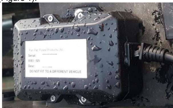
Figure 1: Navman GPS unit mounted on the CAT 552 felling machine.
