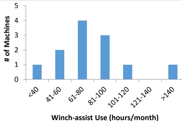
**Figure 6: Monthly hours of use for 12 surveyed winch-assist machines.**
