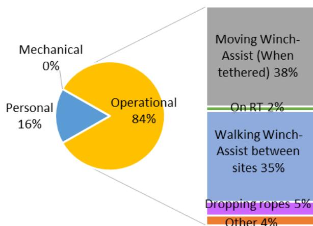
**Figure 8: Types of delays observed during the three day delay study.**
