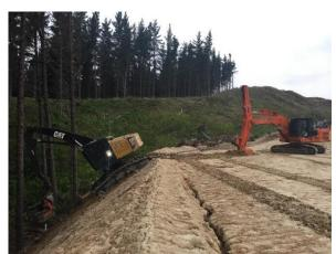
Figure 3: Tractionline winch-assist and CAT 552 felling machine.
