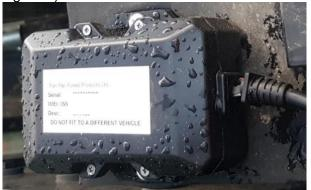
Figure 1: Navman GPS unit mounted on the CAT 552 felling machine.
