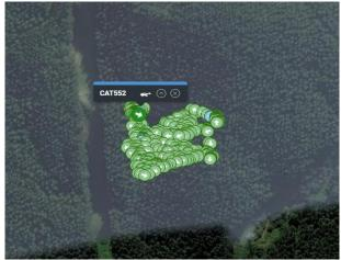
Figure 2: Navman user interface showing felling machine movements for one day's work.
