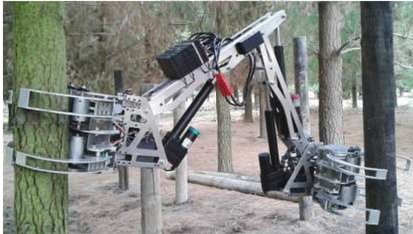
Figure 5: Prototype tree-to-tree machine
