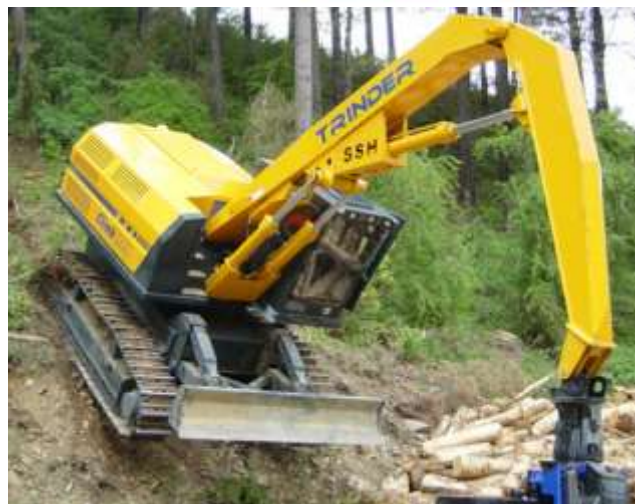
Figure 1: Commercial model ClimbMAX Steep Slope Harvester
