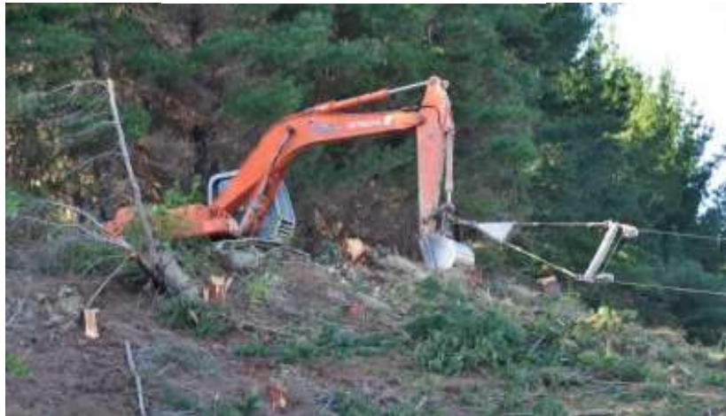
Figure 4: Mobile tail hold machine for CAB system
