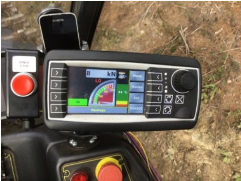
Figure 7. Winch control and display in the harvester.
