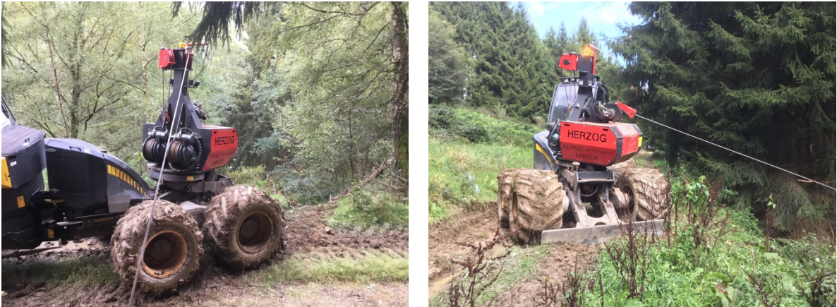
Figure 10. During observations, the winch was used both with one guyline ( left ) and no guylines ( right ). The dozer blade was engaged for additional security.
