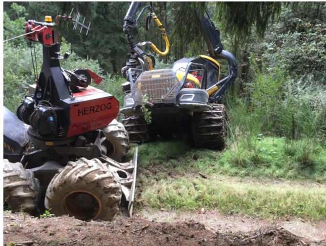
Figure 5. Winching the harvester onto the road. The harvester's boom and cab have been rotated uphill for extra stability.
