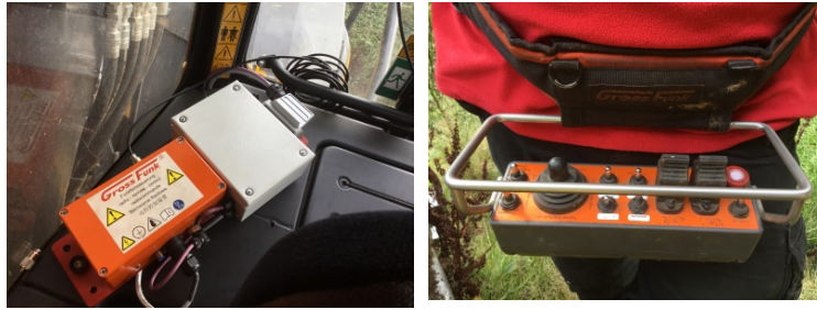
Figure 4. Remote control system for driving the winch machine and operating the guyline winches.
