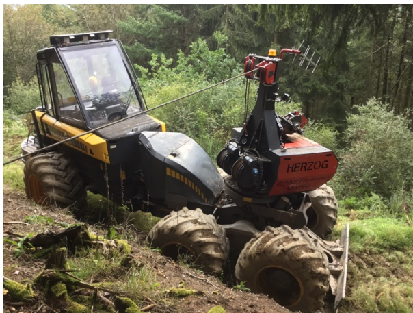
Figure 1. The harvester boom is removed, and the winch system is mounted on the crane's rotating and tilting base.
