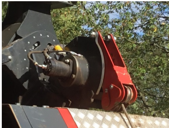
Figure 3. Traction line fairlead is 2.5 m high.
