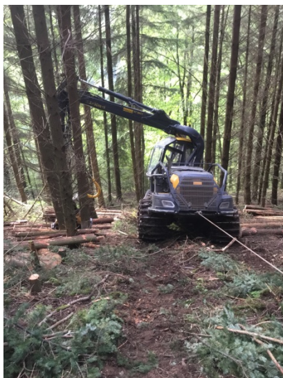
Figure 8. Assisted machine was an eight-wheeled Ponsse ScorpionKing harvester.
