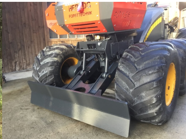
Figure 2. A blade is added to the base of the winch machine for better anchoring.
