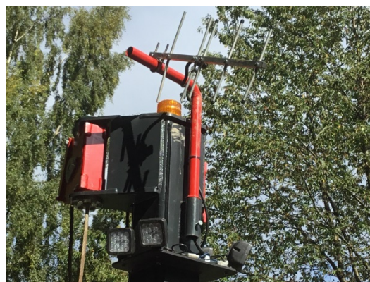
Figure 6. Directional antenna for radio control of the winch system.
